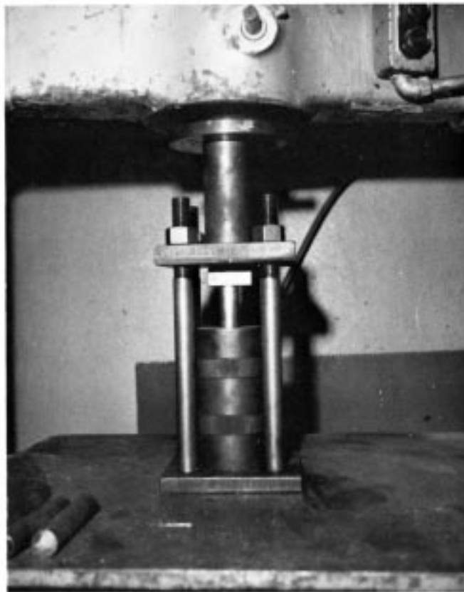
FIG. 3 A Typical Assembled Pressure Vessel
