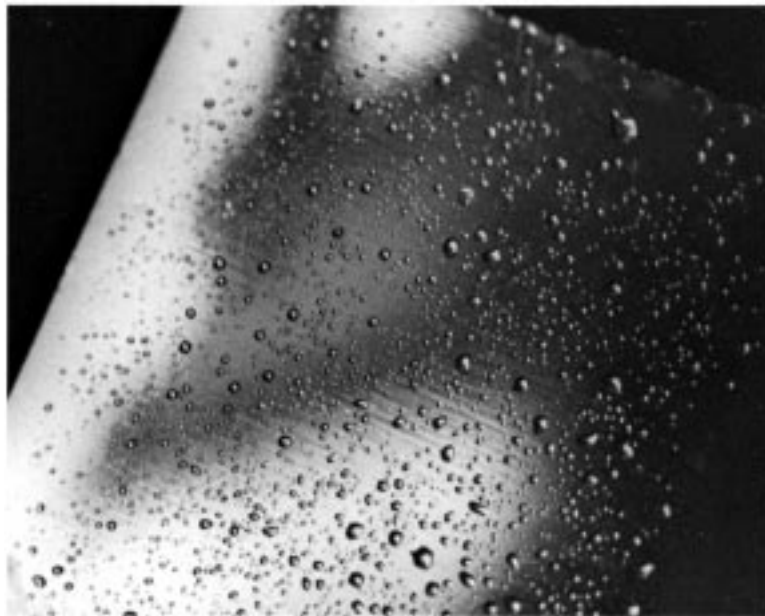
FIG. 5 Atomizer Test of Nickel Specimen with Hydrophobic Film Covering Surface ( \times 2 , Reduced One-Half in Reproduction)
