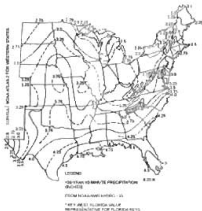
FIGURE 1108.4 RAINFALL RATES FOR PRIMARY ROOF DRAINS (IN/HR)
