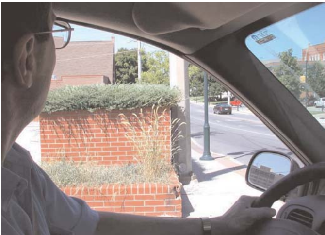
Exhibit 5-4. Placement of planter and utility pole limit the sight distance for a driveway exit.
