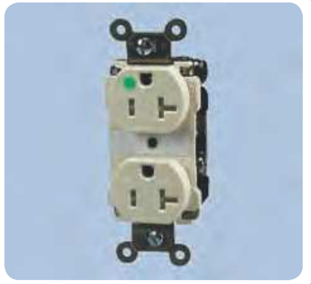
EXHIBIT 517.2 A tamper-resistant hospital-grade receptacle, identified by a green dot on its face, that fulfills the requirements of 517.18(B) and (C). (Courtesy of Legrand/Pass & Seymour®)
