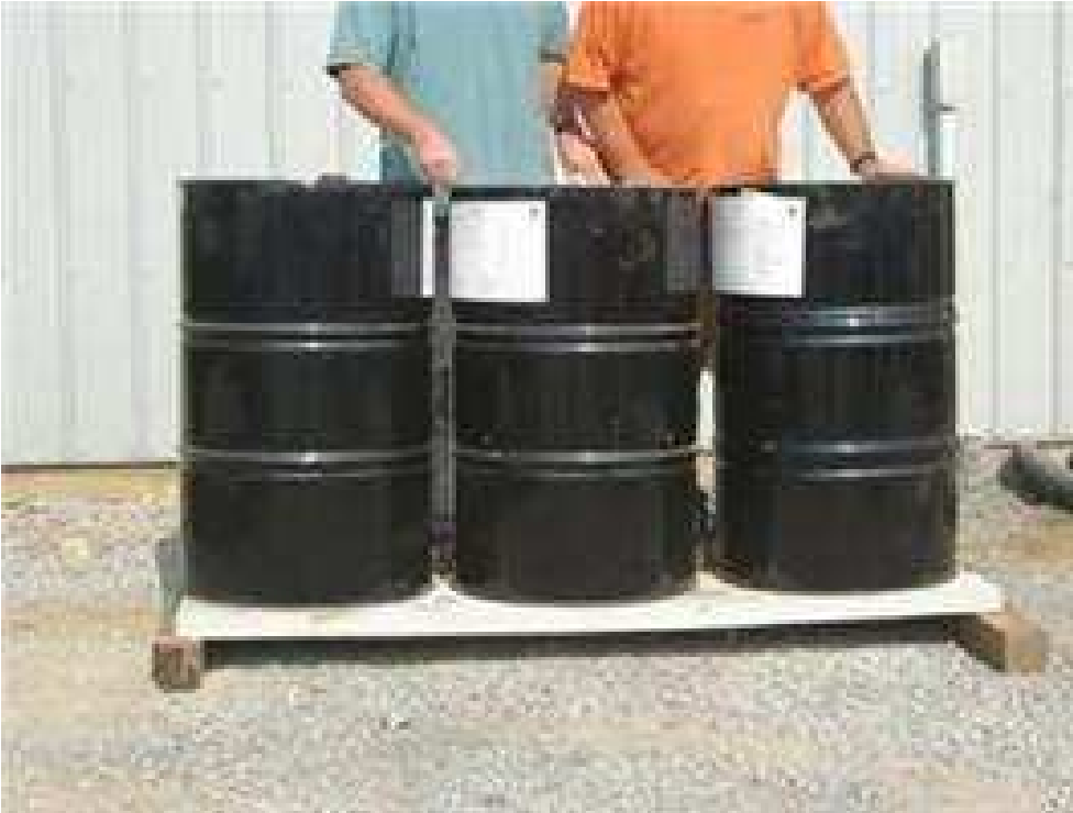
A post-tensioned countertop can support a lot of weight.
