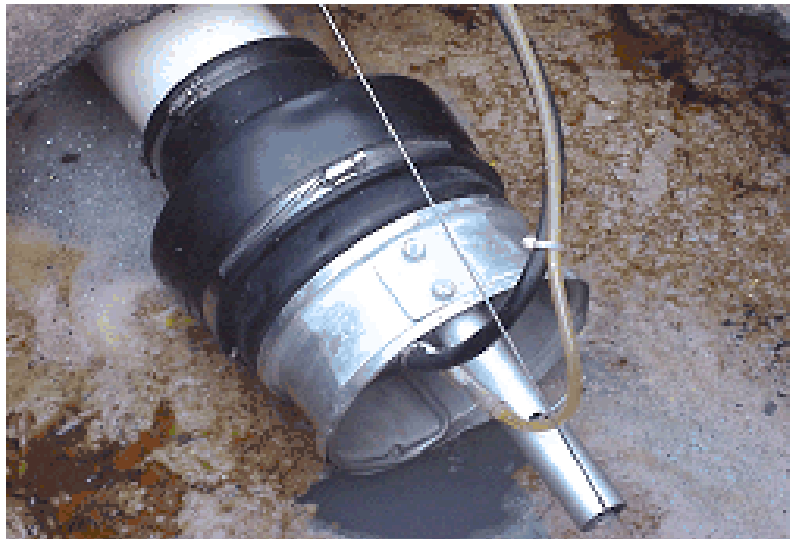
Figure 2-1. V-notch ISCO/Teledyne Flow-Poke Flow Measurement Device in GI.
