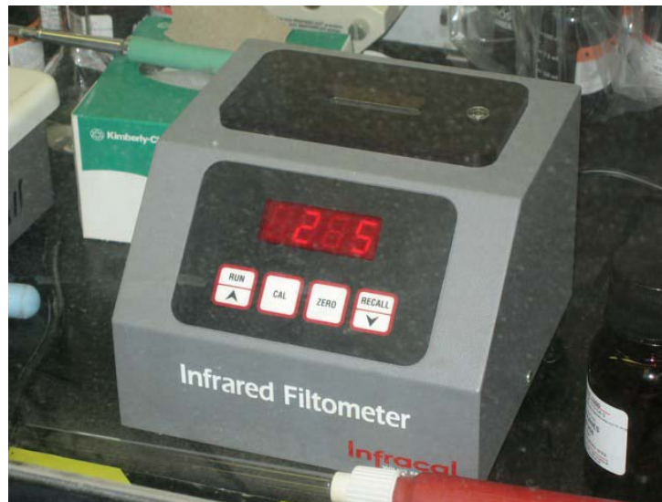
Figure 2-10. Infracal ® Device Used for FOG Concentration Measurements.
