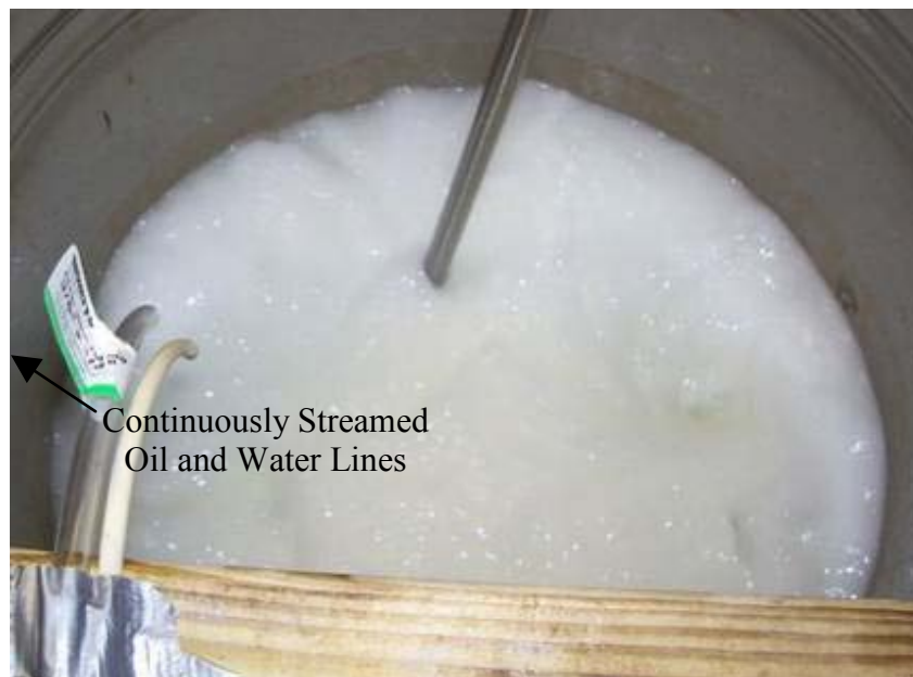
Figure 2-5. Oil/Water Mixing Drum.
