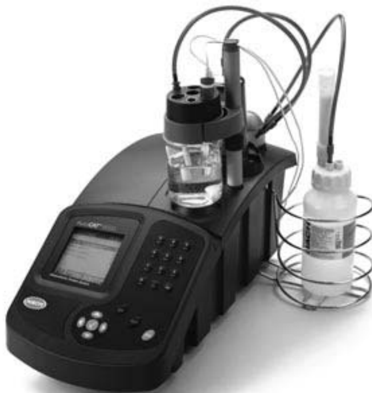
Figure 2.4: Hach Company’s AutoCAT 9000 Amperometric Titrator
