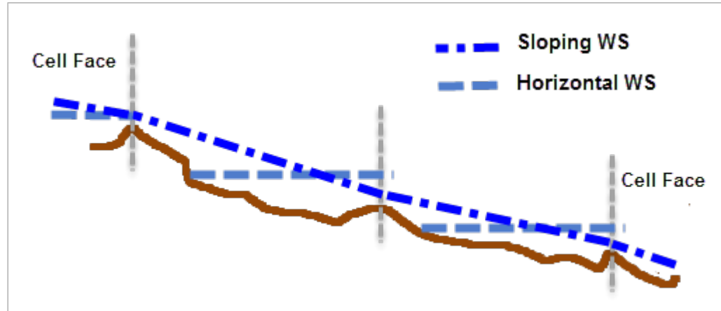
Figure 20-32. Comparison of Sloping and Horizontal water surface rendering.
