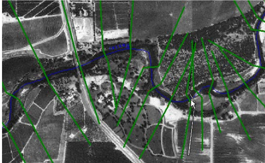
Figure 6-122. The bridge sections are upstream of the real world location.
