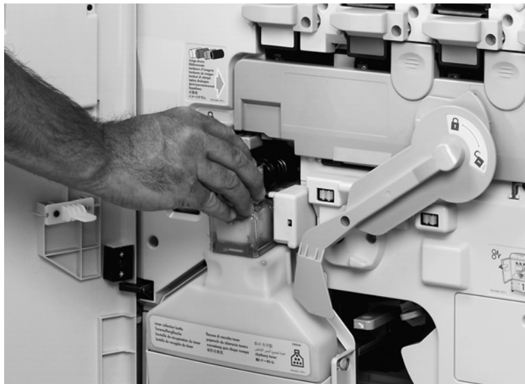
Figure 81. Remove the waste toner bottle
