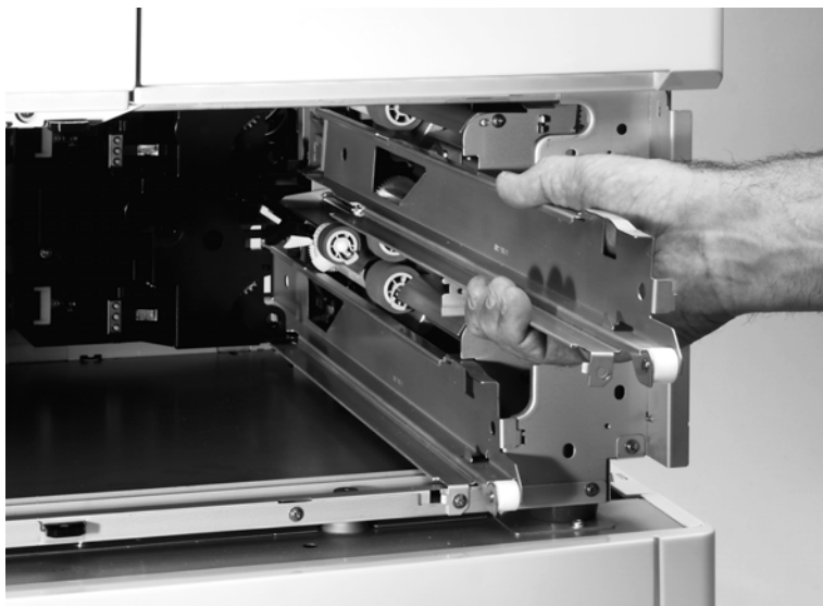
Figure 196. Remove the tray guides
