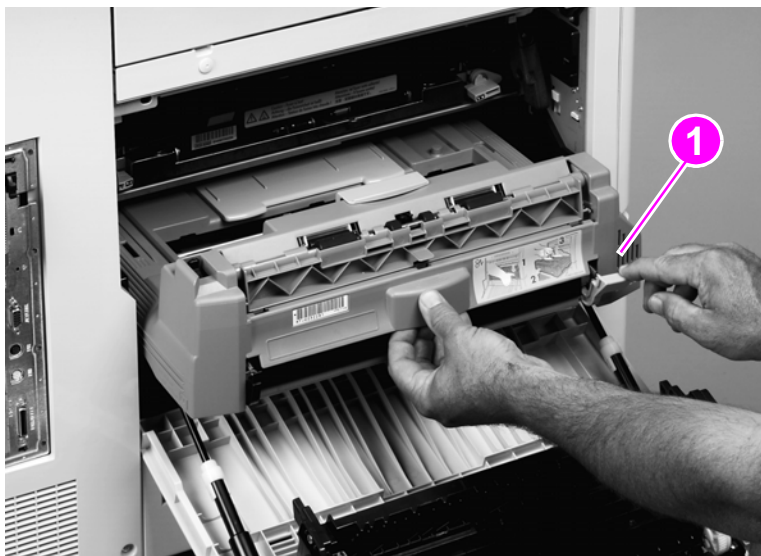
Figure 160. Remove the duplexer
