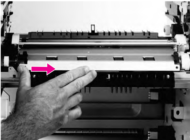
Figure 213. Remove the registration assembly plate (1 of 2)
