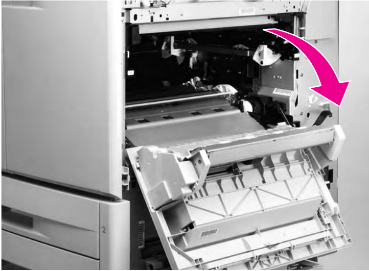
Figure 107. Open the ITB door
