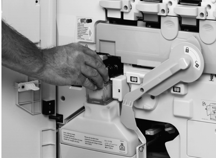
Figure 81. Remove the waste toner bottle
