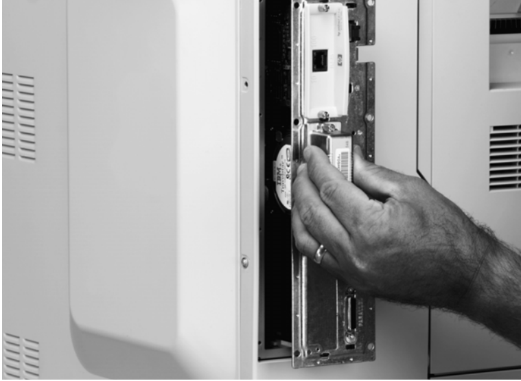
Figure 234. Remove the formatter PCB
