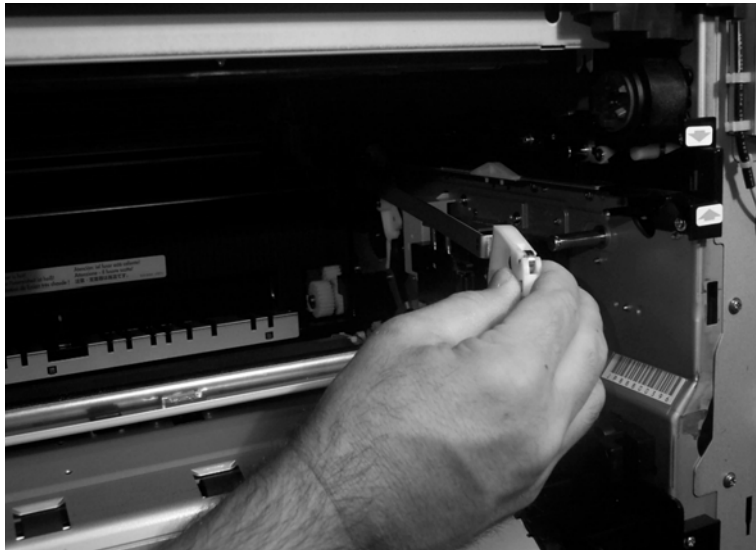
Figure 222. Remove the right back ITB lift link (2 of 2)
