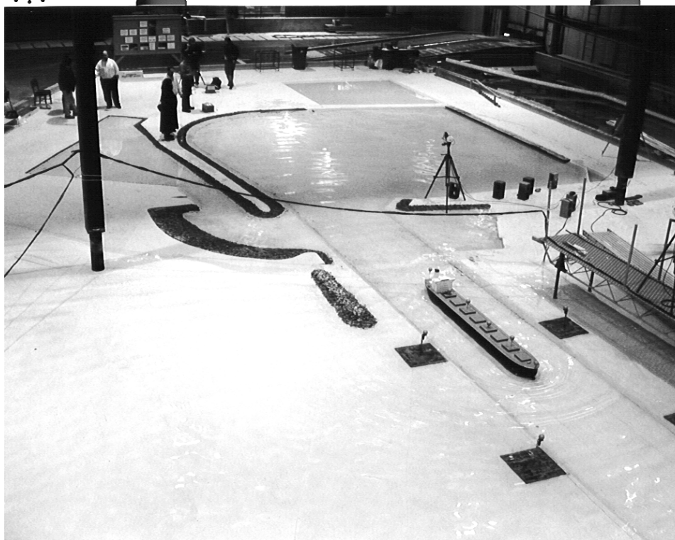
Figure V-5-57. Physical model of Barbers Point Harbor
