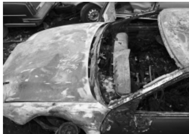
FIGURE 22.8(f) Radial pattern on the passenger side door produced by an engine compartment fire.
