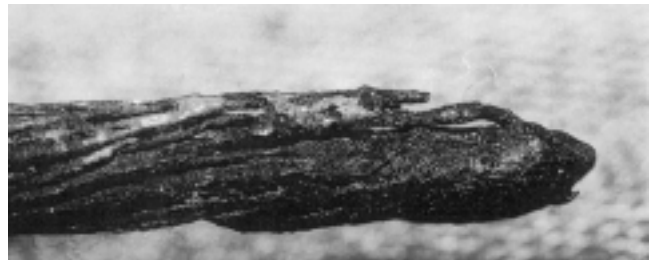
FIGURE 6.10.6.2(e) Another example of fire melting of stranded copper wire.
