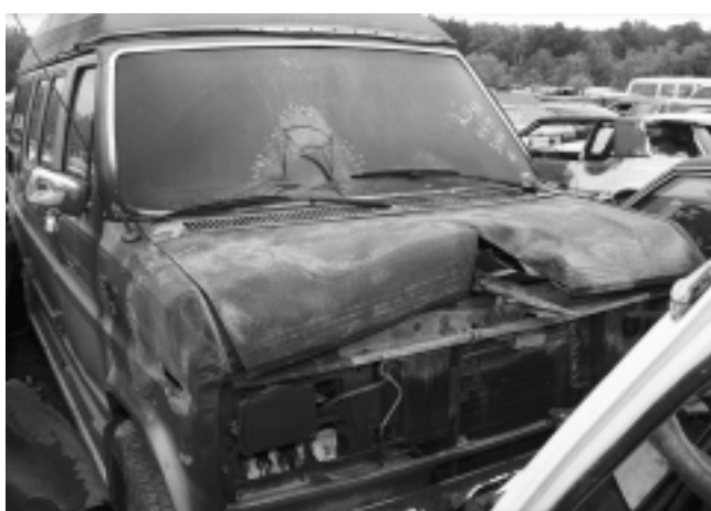
FIGURE 22.8(e) Incipient windshield failure caused by an engine compartment fire.
