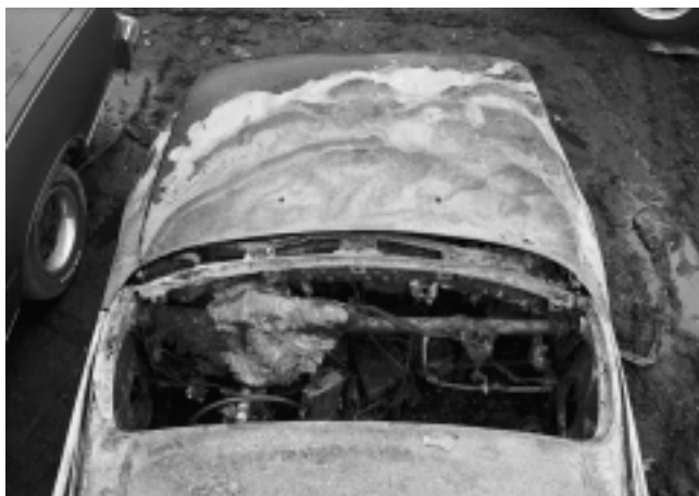
FIGURE 22.8(d) Radial burn pattern produced by a passenger compartment fire.
