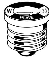
FIGURE 6.6.1(a) A typical, Edison-based nonrenewable fuse, single element, for replacement purposes only.
