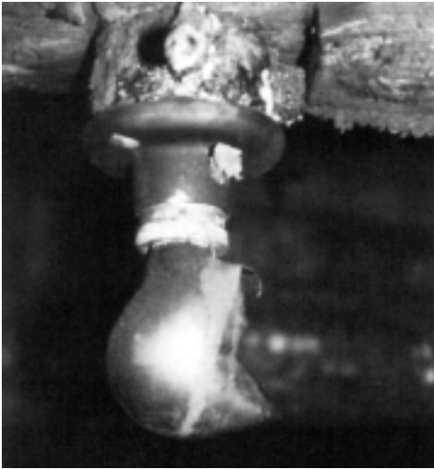
FIGURE 4.20.1 A typical “pulled” bulb showing that the heating was from the right side.
