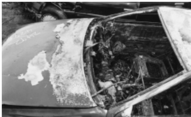
FIGURE 22.8(c) Radial burn pattern produced by a passenger compartment fire.
