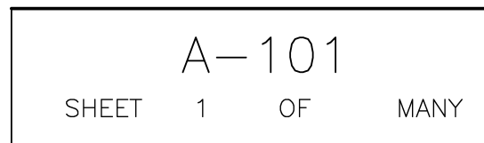
Figure 02.10 Sheet identification block.
