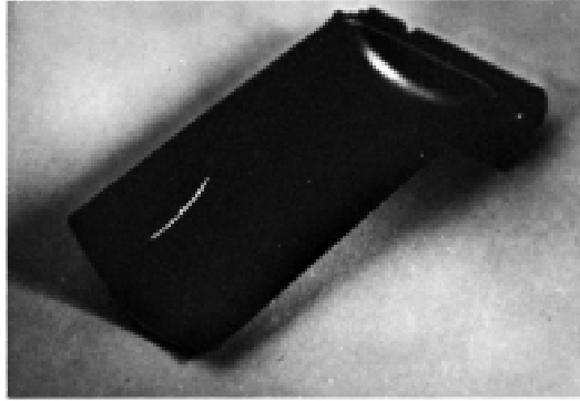
FIG. 5 Example of Type II, Class A, Indication
