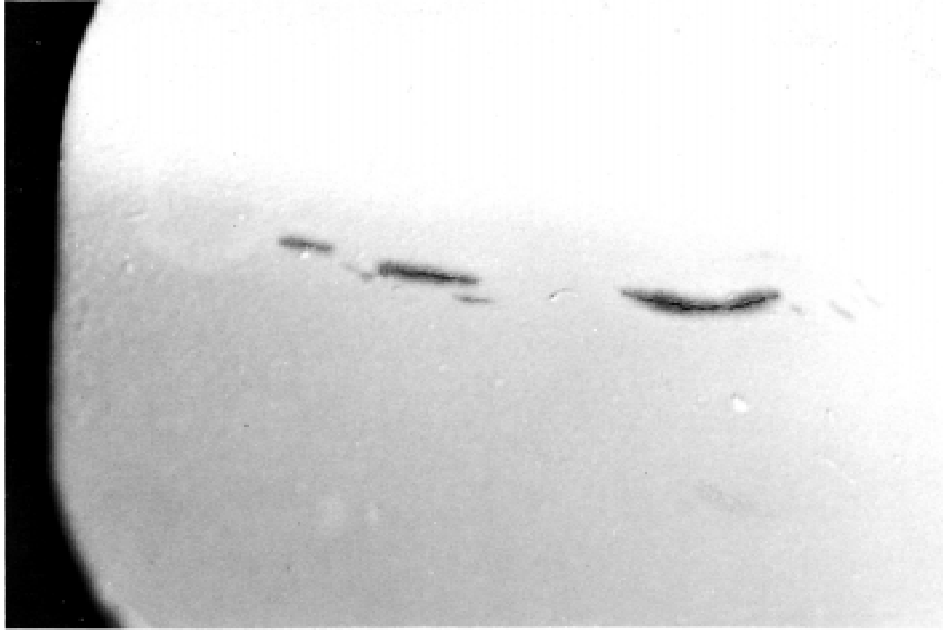
FIG. 7 Example of Type II, Class C, Indication
