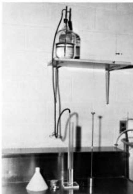
FIG. 4 Graduated Cylinder, Irrigator Tube, Weighted Foot Assembly, and Siphon
