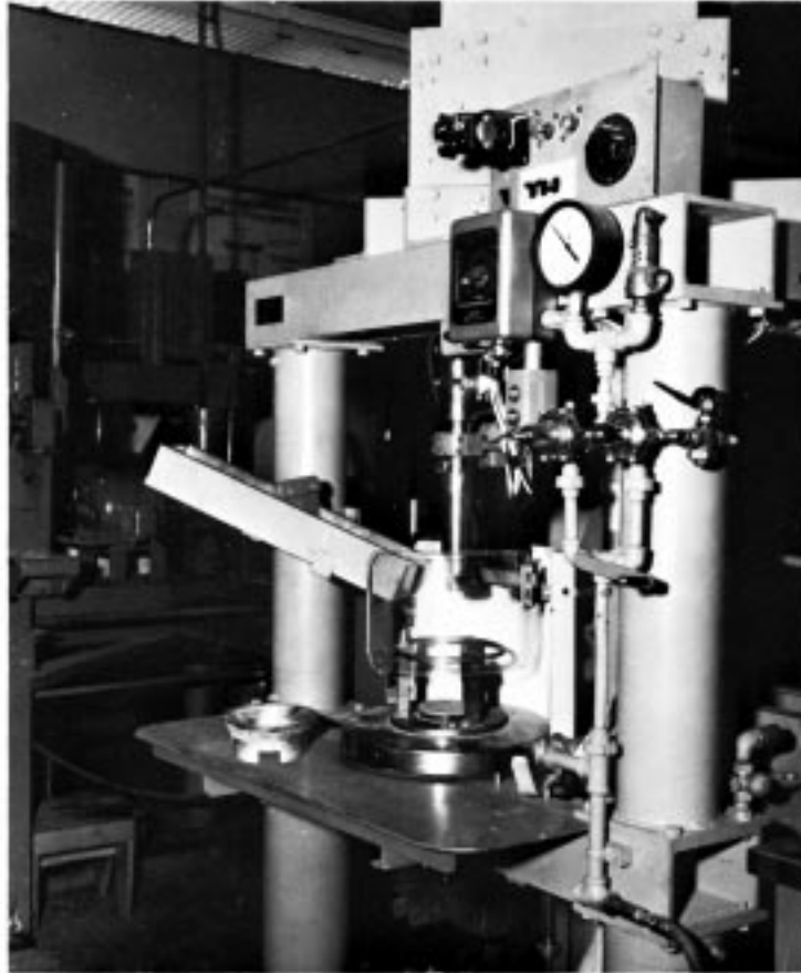
FIG. 2 Compactor with Sample Feed Trough
