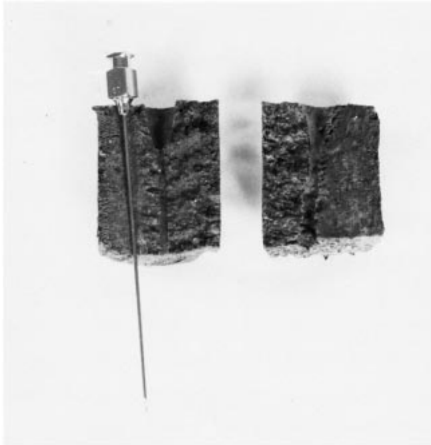
FIG. 4 Appearance of Typical Clay Pinhole Specimens After Completion of Test
