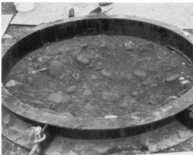
FIG. 4 Test Pit During Excavation
