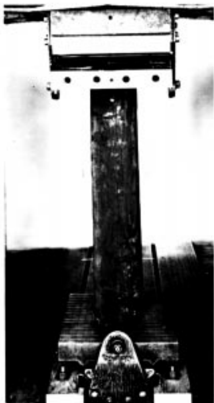
FIG. 5 Compression of a Wood Structural Element
