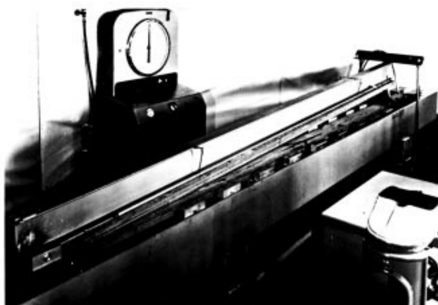
FIG. 7 Compression of Long Slender Structural Member
