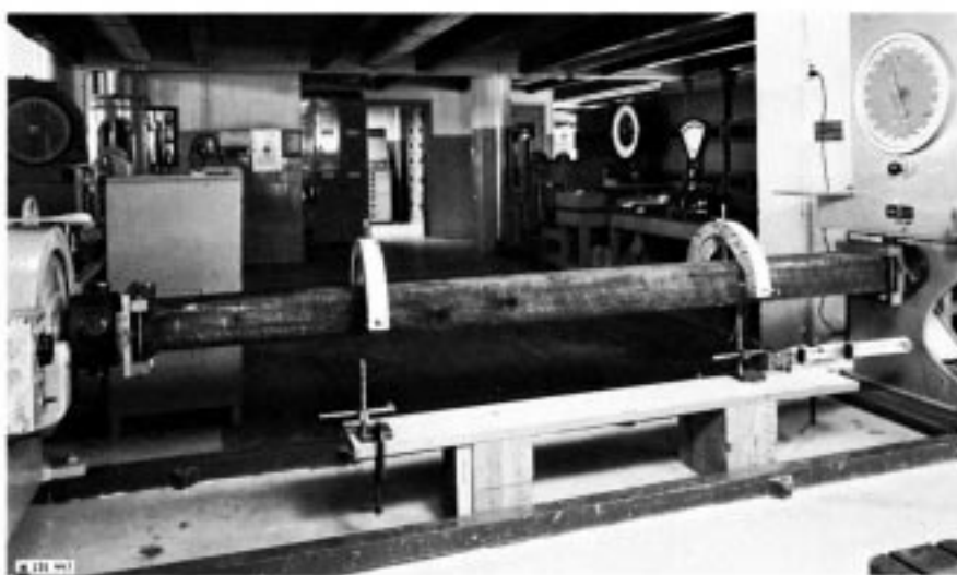
FIG. 15 Torsion Test with Yoke-Type Troptometer
