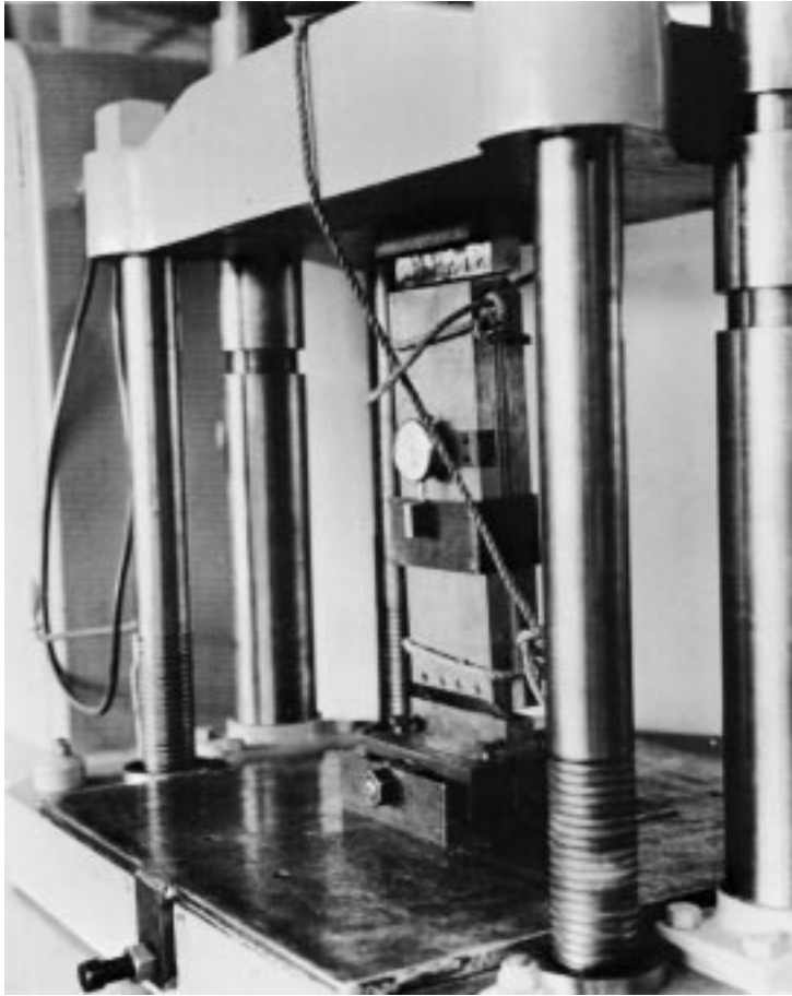
FIG. 3 Planar (Rolling) Shear Specimen Ready for Testing
