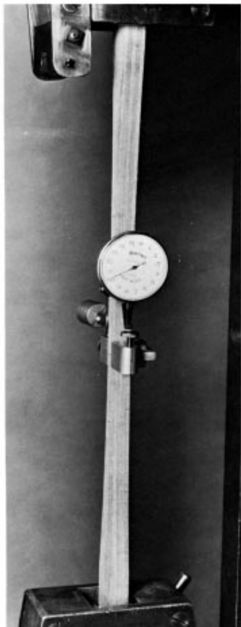
FIG. 2 Tension Test of Thick Plywood Showing Nonaveraging Type of Extensometer (2-in. Gage Length)
