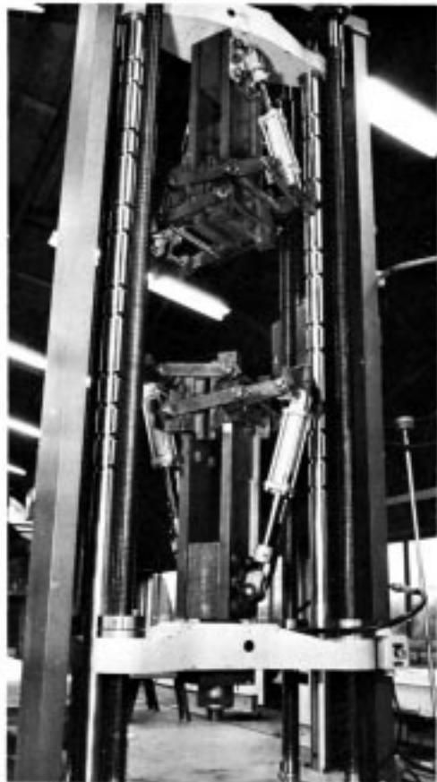
FIG. 5 Grips Suitable for Test Method B Tension Tests
