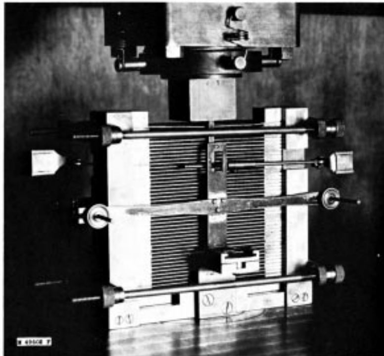
FIG. 1 Compression Test of Thin Structural Panel Supported Laterally Showing Marten's Mirror Compressometer for Measuring Deformations on Two Opposite Faces
