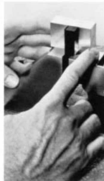
FIG. 4 Jig for Positioning Specimen for Clamping
