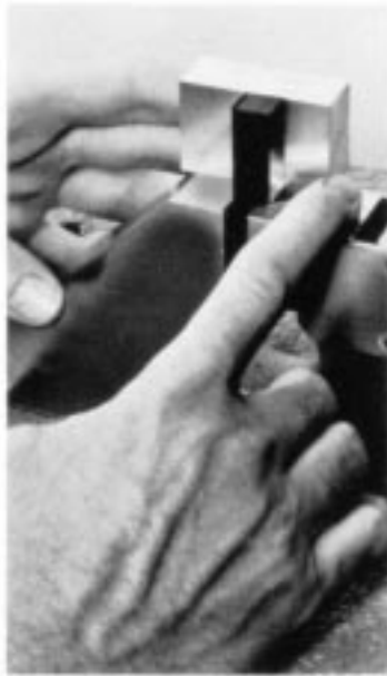
FIG. 4 Jig for Positioning Specimen for Clamping
