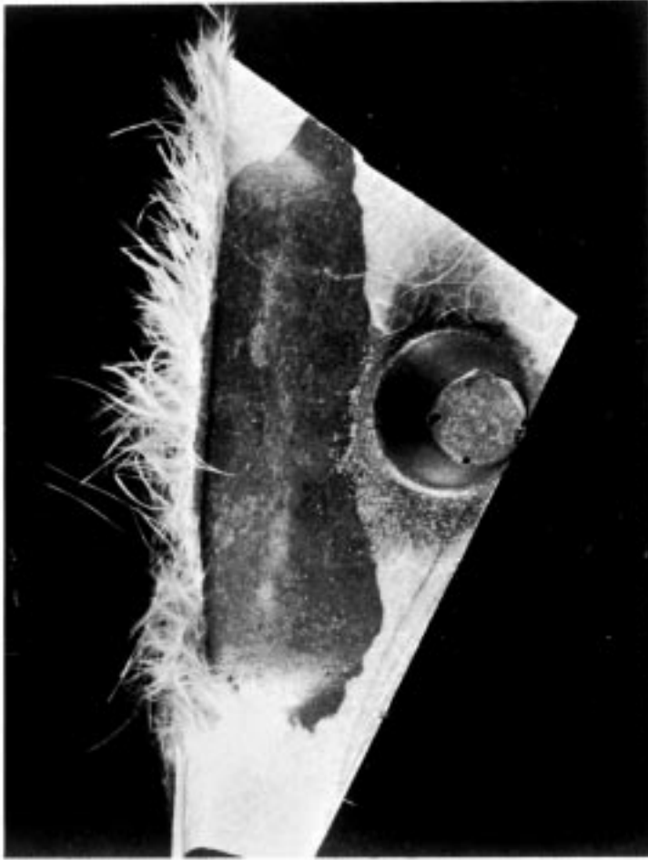
FIG. 11 Lack of Fillout
