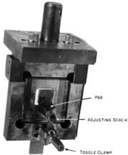
FIG. 6 Rear View of Fixture with Specimen Clamped in Place
