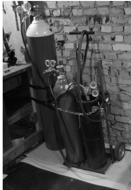
Figure 202-H5 TYPICAL WELDING CART
