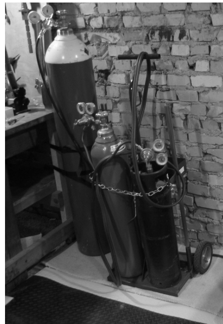
Figure 3505.2.1 TYPICAL WELDING CART
