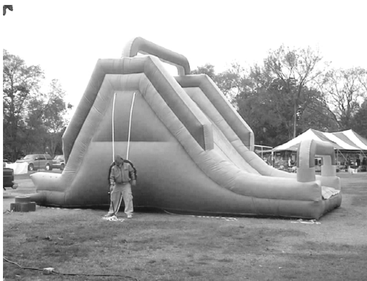
Figure 202-A1 EXAMPLE OF AIR-INFLATED MEMBRANE STRUCTURE
