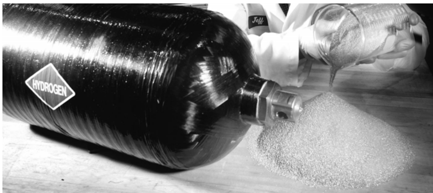
Figure 202-M1 METAL HYDRIDE STORAGE CONTAINER AND ITS METAL HYDRIDE CONTENT Photo courtesy of Ovanics Hydrogen Systems, LLC
