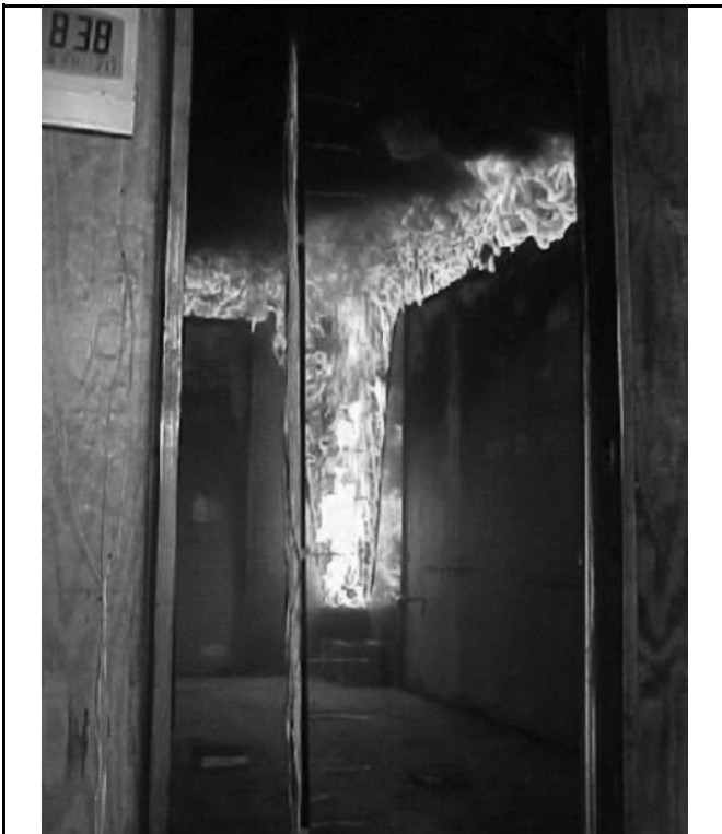
Figure 803.1.2(2) FLAME IN ROOM CORNER TEST
