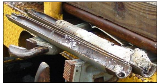
Figure 1: Split spoon SPT sampler
