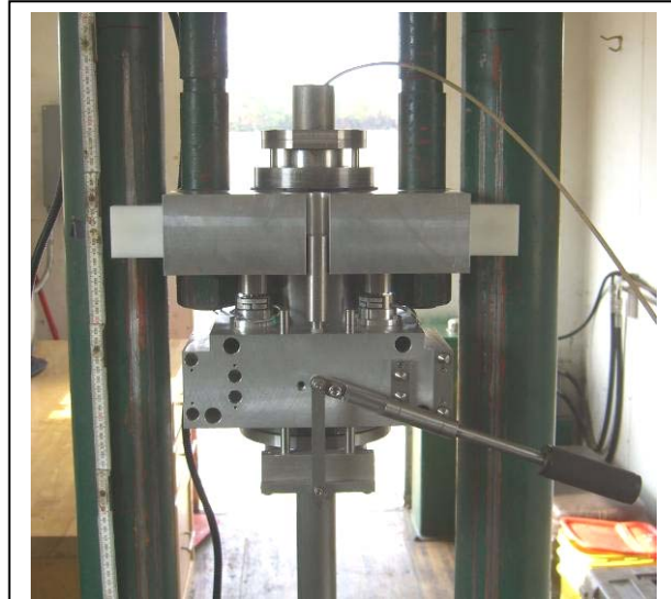
Figure 5: Push Clamp using Four Load Cells to Measure Thrust
