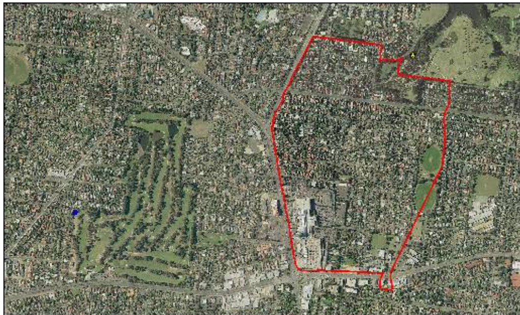
Figure 3-17 Aerial photo of Doncaster catchment, with the Eastern Golf Club (and alternate rain gauge shown by the blue dot) visible on the left of the photo. The yellow dot in the top right shows the flow, pollutant and rainfall gauge
