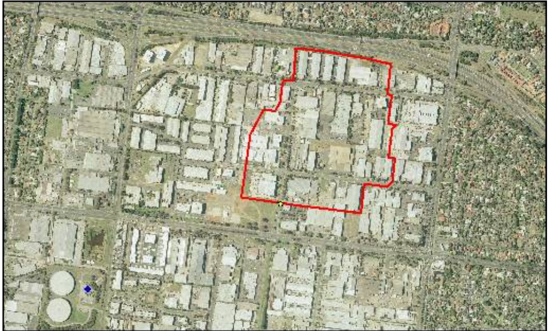
Figure 3-6 Aerial photo of the Mt. Waverley catchment, with the Melbourne Water Notting Hill rain gauge position shown at the bottom left of the photo. The blue dot shows the location of the rainfall gauge and the yellow star the flow/pollutant monitoring point
