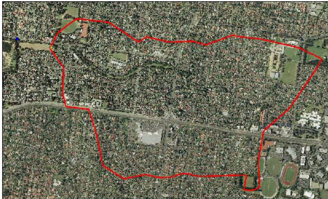
Figure 3-14 Aerial photo of the Burwood East Catchment with catchment boundary. The flow and pollutant sampling point is shown by the yellow star. The blue dot is the alternate monitoring point and the one-minute rainfall monitoring point is on the right hand boundary of the photo
