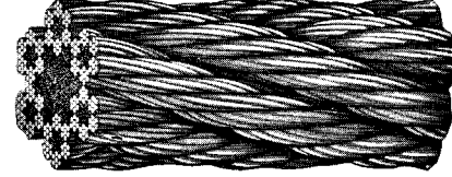
6 x 42—7 Fiber Cores—Tiller Rope
