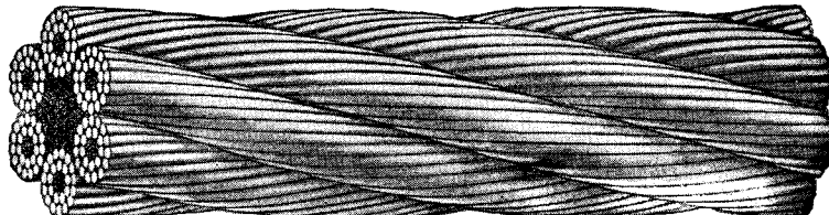
6 x 24—7 Fiber Cores—Galvanized Mooring Line
