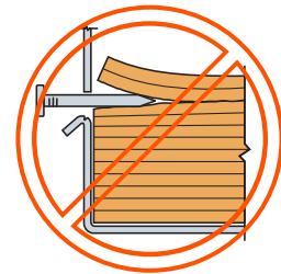
Nail at wrong angle
