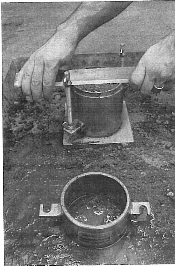
Figure 12.4. Excess soil being trimmed (Step 8).
