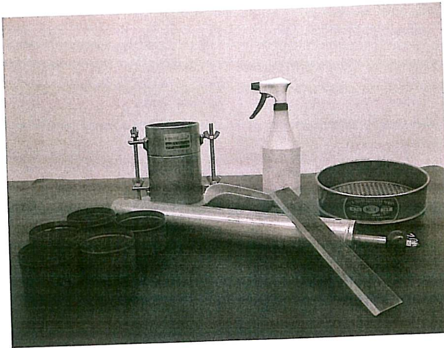
Figure 12.1. Equipment for Proctor compaction test.
