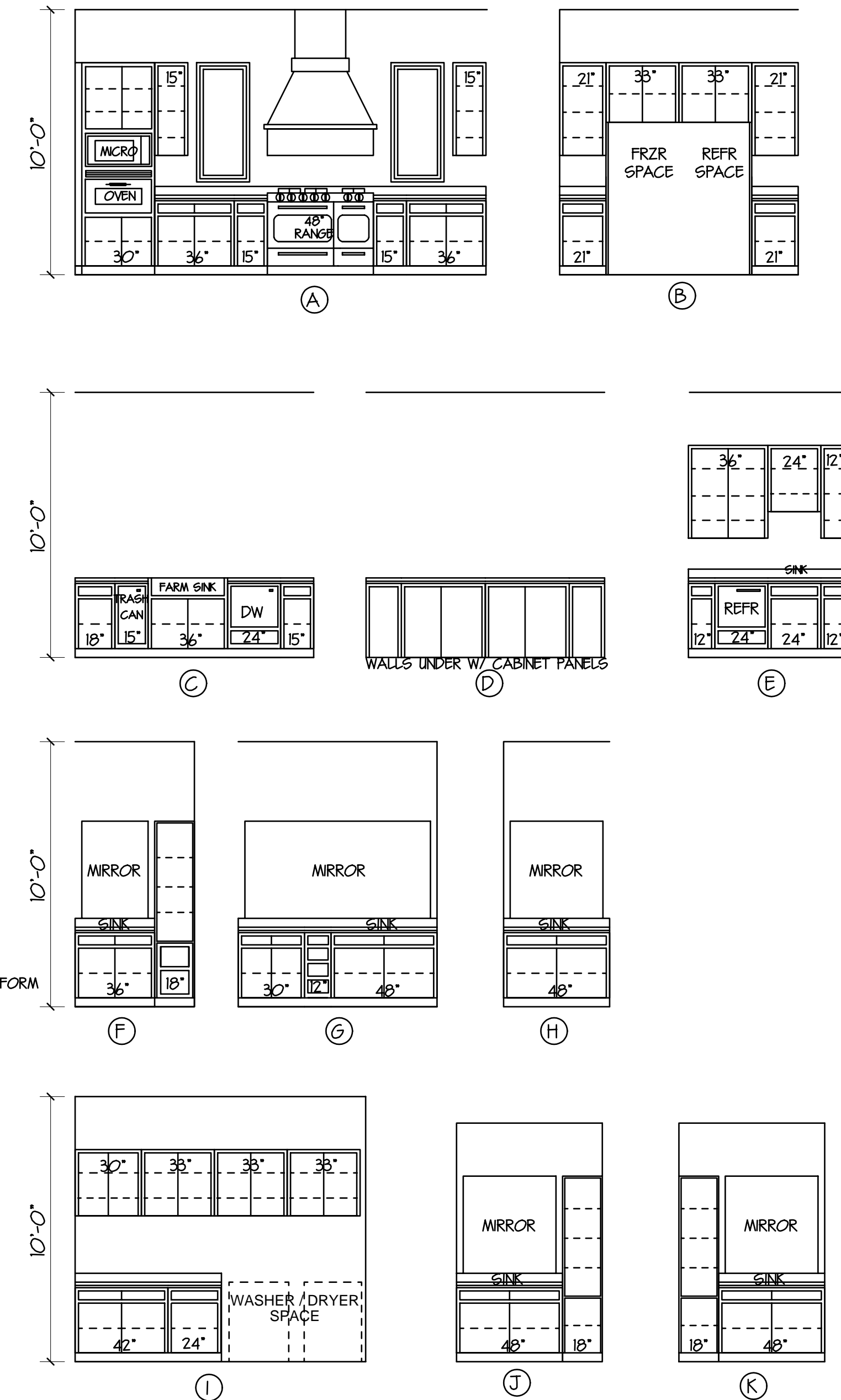
CABINET ELEVATIONS SCALE 1/4" = 1'-0"
