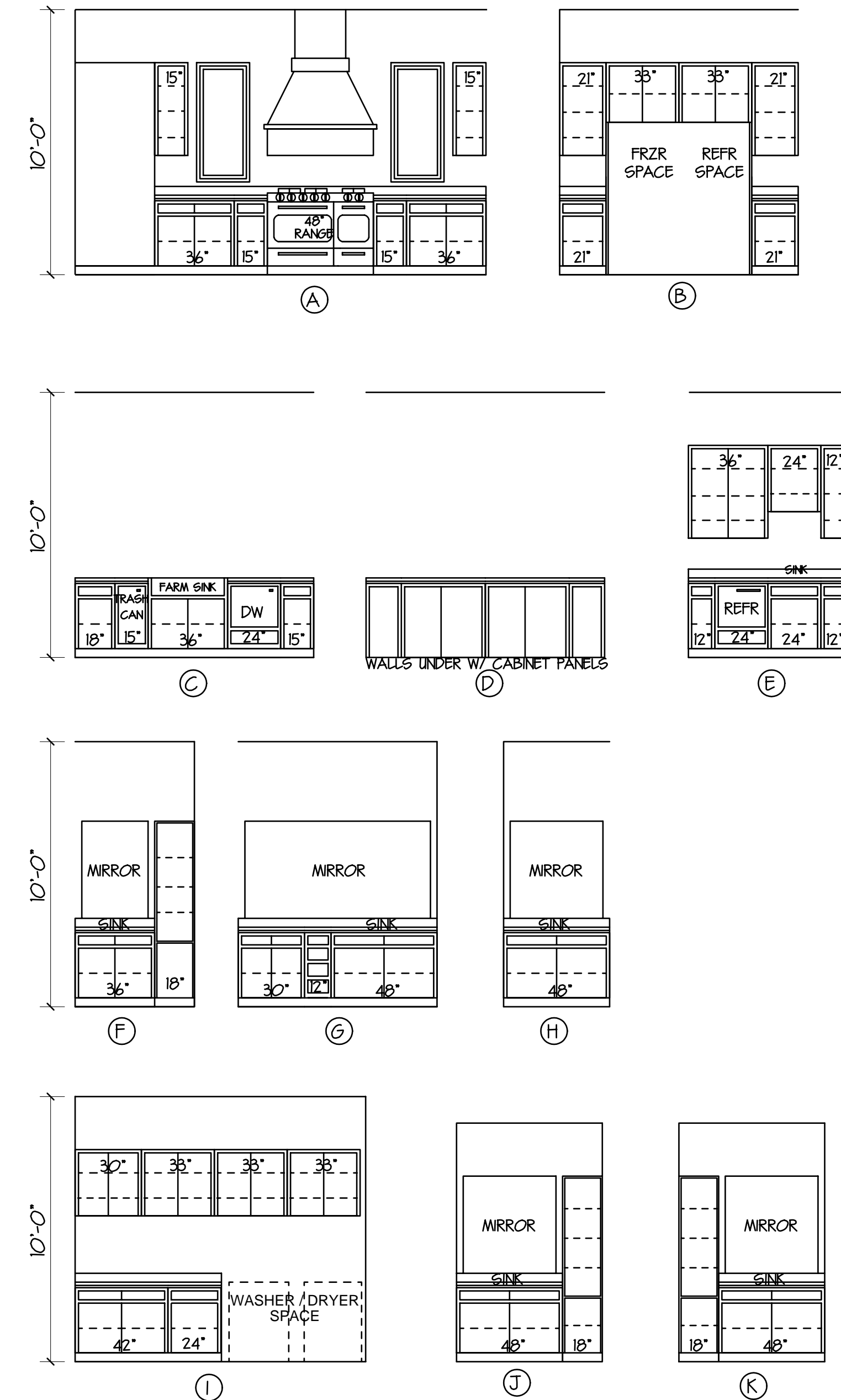
CABINET ELEVATIONS SCALE 1/4" = 1'-0"
