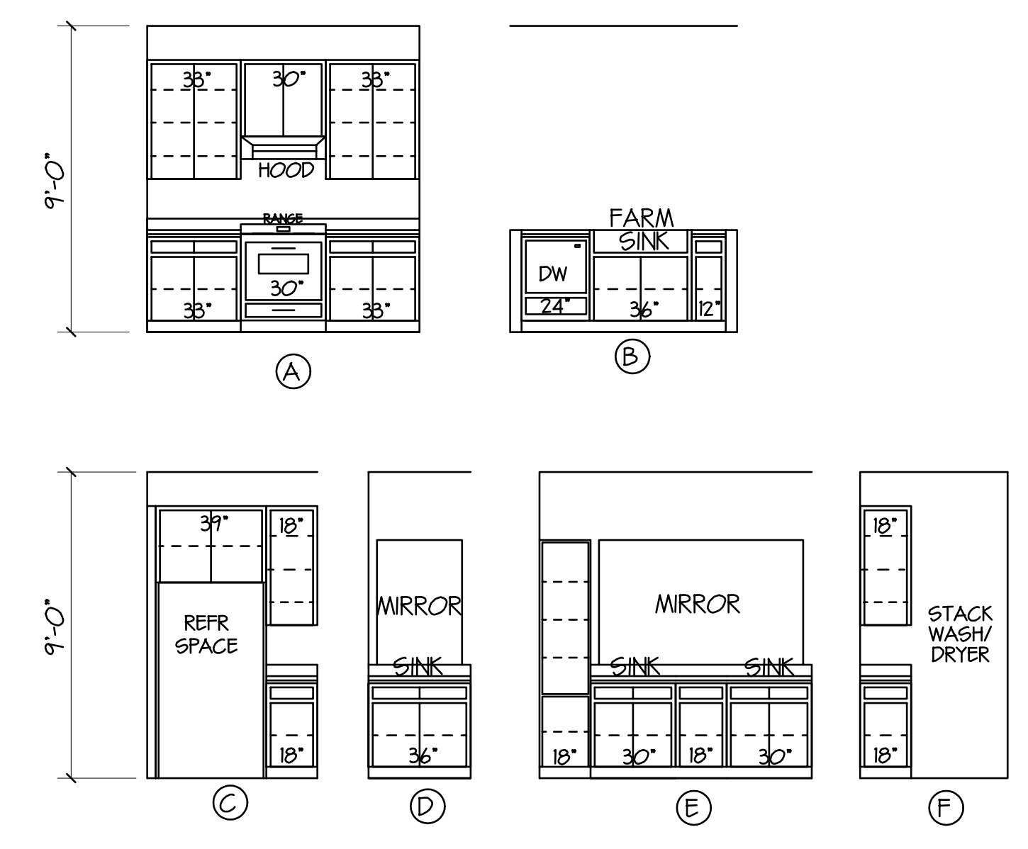
CABINET ELEVATIONS SCALE 1/4"=1'-0"
