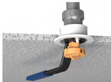
Figure 4: Recessed Installation (with standard Installer's Wrench)
