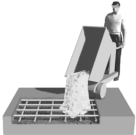
Fig. 8—Place repair material into the prepared cavity by buggy, pump, or other conveying method.
