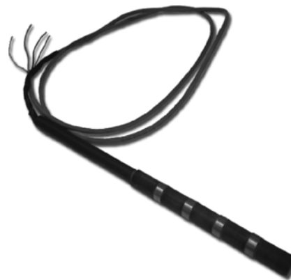
Fig. 1—Electrical resistivity probe developed in this study. (Note: Electrode spacing is 1 in. [2.5 cm].)
