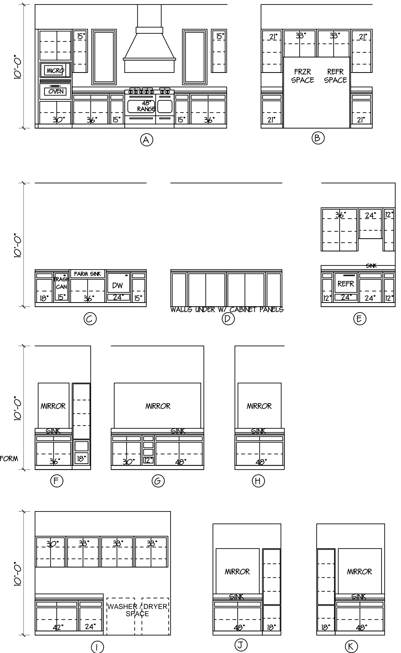
CABINET ELEVATIONS SCALE 1/4" = 1'-0"
