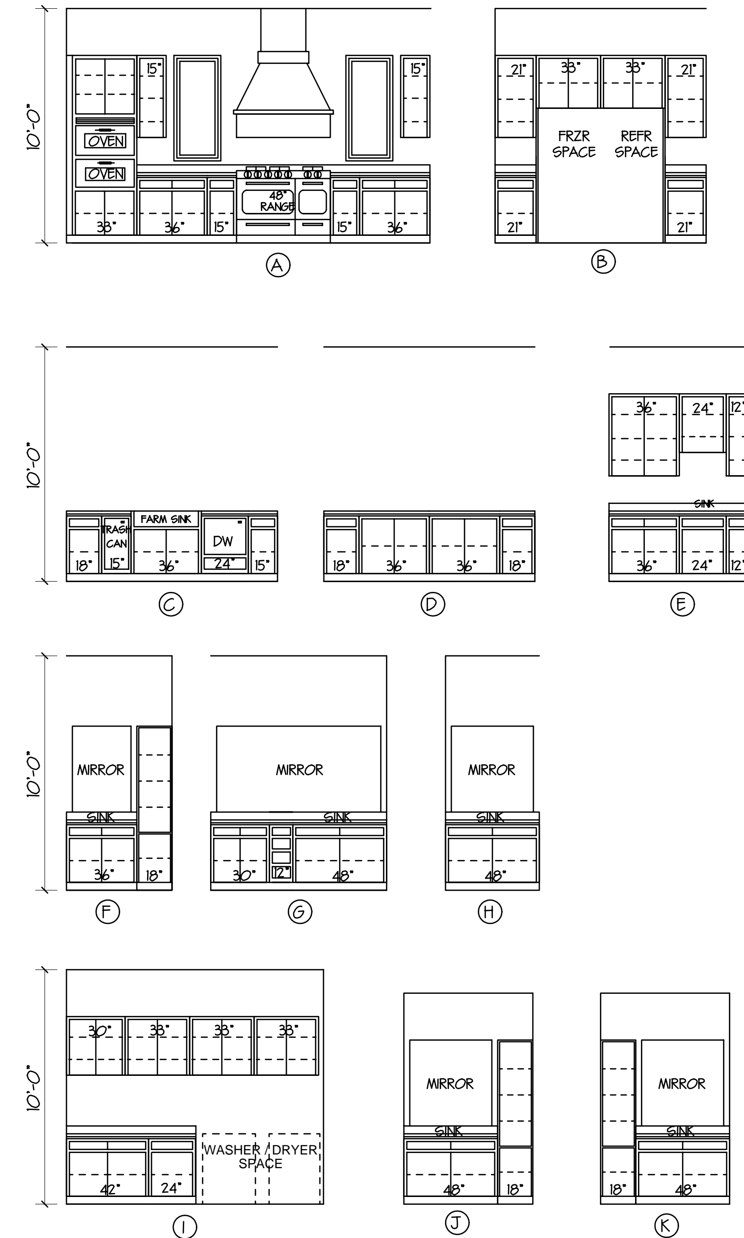
CABINET ELEVATIONS SCALE 1/4" = 1'-0"
