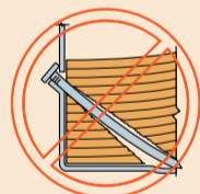
Nail Too Long
