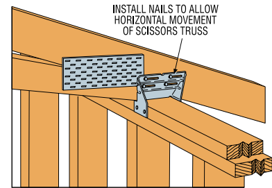
Typical TC24 Installation
