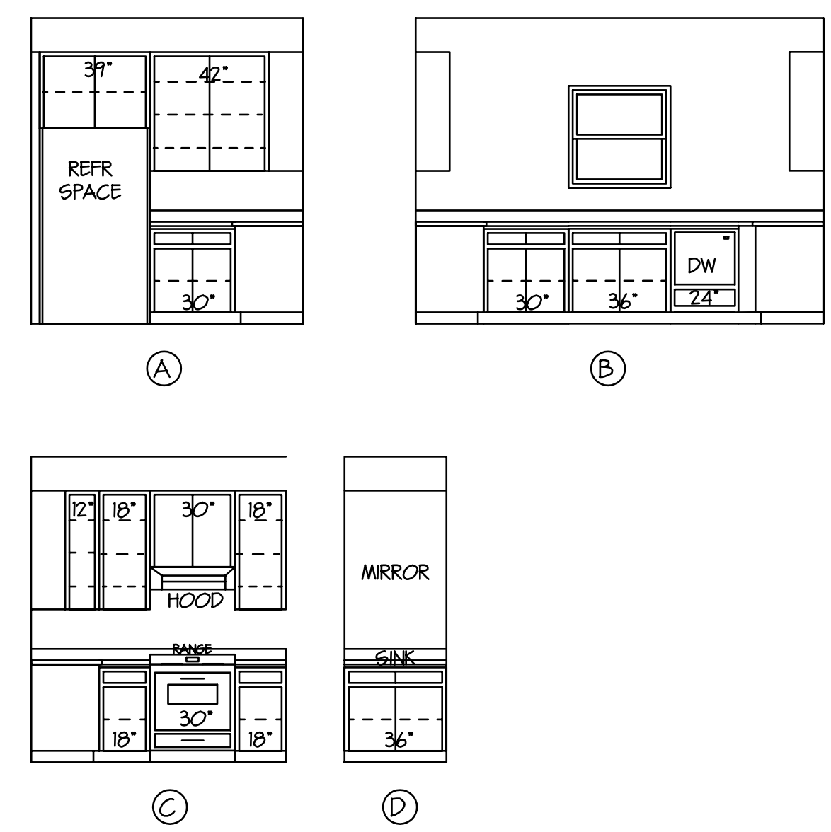
CABINET ELEVATIONS SCALE 1/4"=1'-0"
