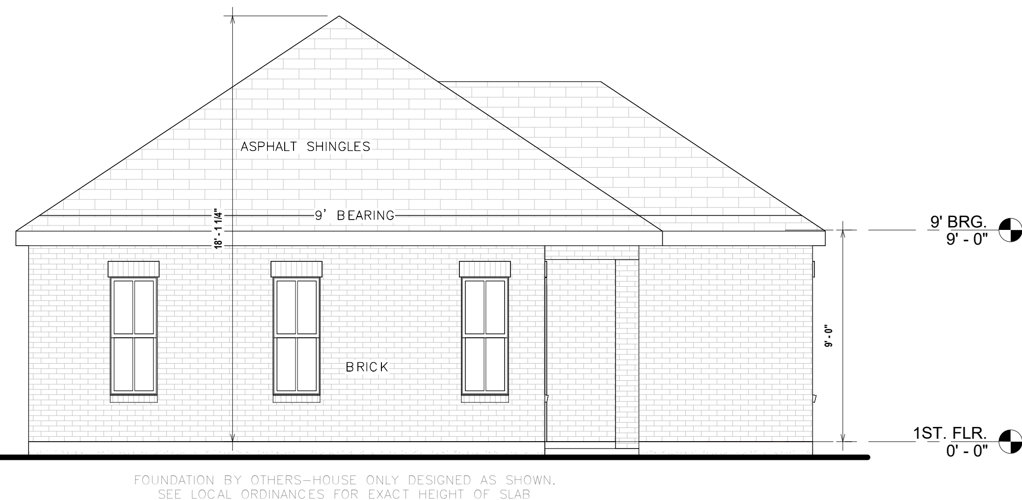
A1 POOL HOUSE LEFT ELEVATION 1/4" = 1'-0"
