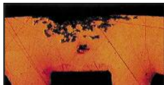
Fig. 2 Formicary Corrosion Tunneling
