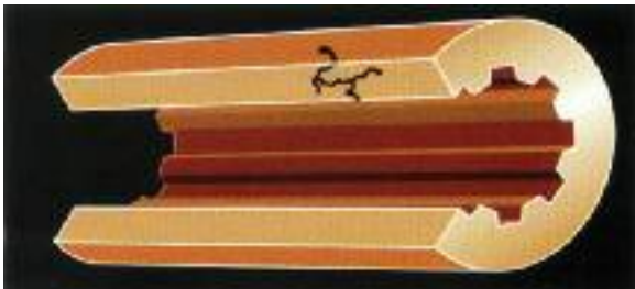
3-D representation of corrosion through tube
