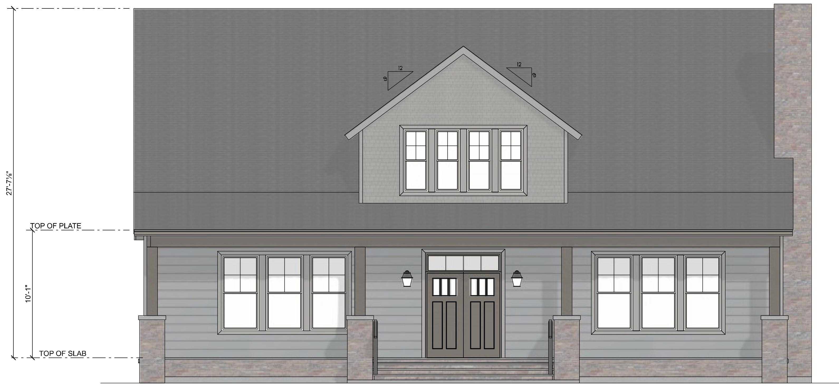
FRONT ELEVATION SCALE = 1/4"=1'-0"
