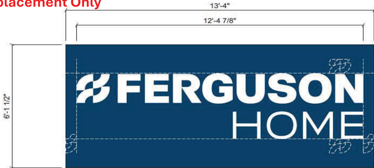
B FRONT VIEW @ REPLACEMENT FACES - Qty.2 Scale: 1/2"=1'
