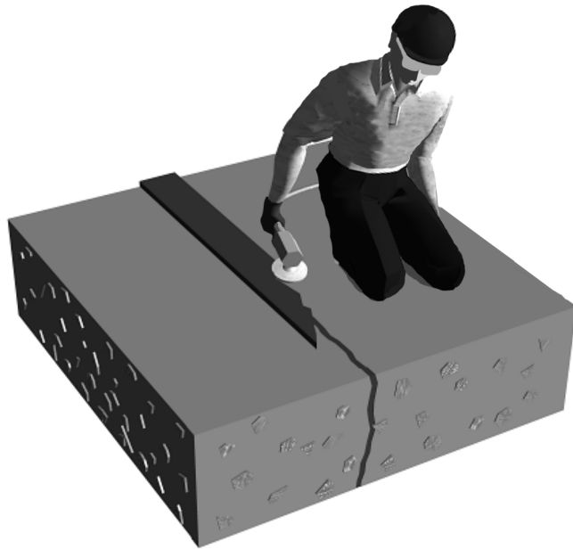
Fig. 6—Remove seal cap.
